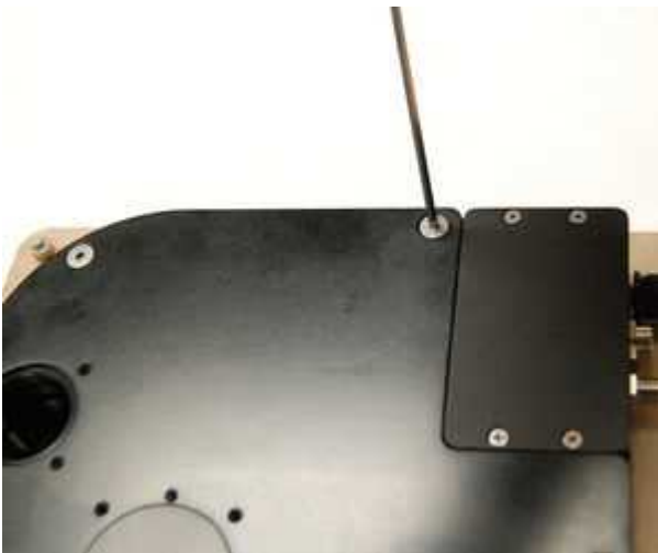
Remove the X-FWR-E housing lid using a 2.5mm hex key to remove the four cover screws.
