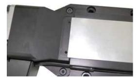
Position the dust cover so it comes close to the clamp holes at each end.
