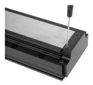
Loosely attach the clamps at each end. Run the stage back and forth once to position the dust cover. Gradually tighten the clamp screws, alternating between the two at each clamp. If part of the dust cover isn't seated properly, loosen the nearest clamp and re-tighten.
