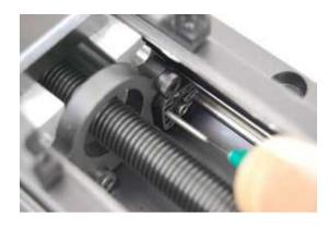
Insert angled syringe tip into grease hole in bearing end cap. With the power on and using the manual control knob (if equipped), move the stage about 100 mm (4") while squeezing grease in from the syringe.
